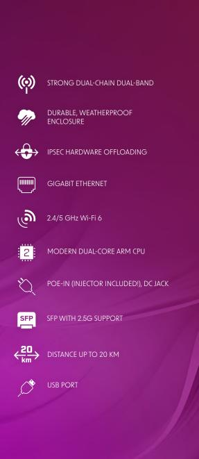
Managing outdoor wireless network has never been easier: mANTBox ax 15s can provide unparalleled wireless point-to-multipoint connectivity for a vast variety of devices over a distance of 20 kilometers!
